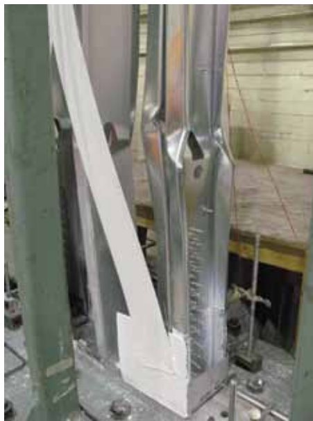
Figure 2: Diagonal strap braced wall with 4:1 aspect ratio. Courtesy of AISI & McGill University.
