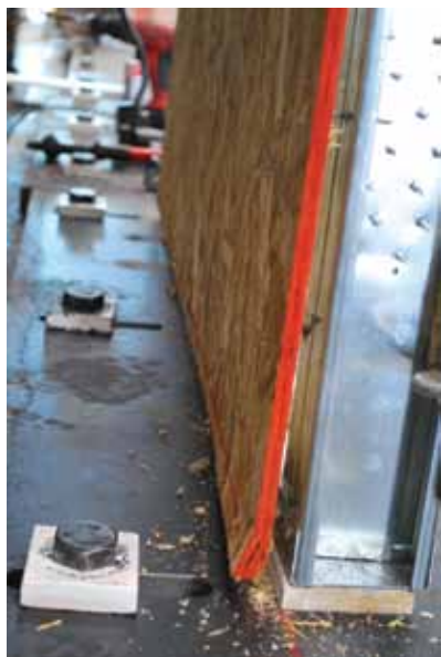
Figure 6: Non-winged self-tapping screw test assembly failure.
