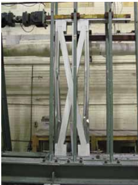
Figure 2: Diagonal strap braced wall with 4:1 aspect ratio. Courtesy of AISI & McGill University.
